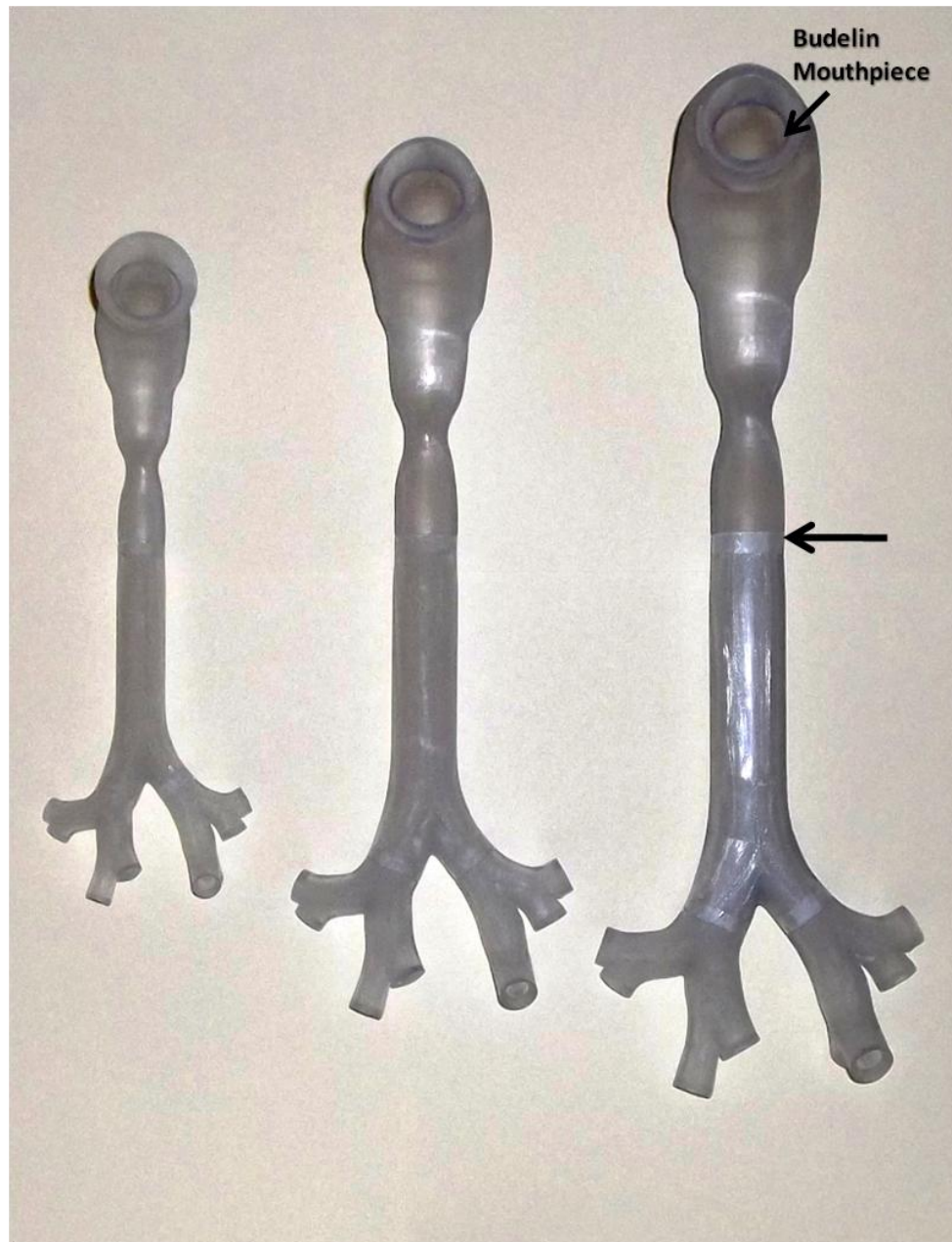
Figure 3.2: The small, medium and large MT-TB models used in the present study. Complete dimensional description is available at http://www.rddonline.com/resources/tools/models.php . Models were constructed of Accura 60 (3D System, Valencia, CA) using rapid prototyping (Viper SLA, 3D Systems). MT models were made to snap fit (at arrow) on top of companion TB models to form MT-TB S , MT-TB M and MT-TB L with internal volumes of MT = 26.6, 61.6, 96.1 and TB = 16.3, 39.0, 61.6 cm 3 , respectively. The integral Budelin mouthpiece adapter added an additional volume of 5.4 cm 3 to all models.
